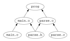
This is an *acyclic* graph because of the arrows which express the ordering of the relationship between the files. If there *was* a circular dependency according to the arrows, it would be an error.
